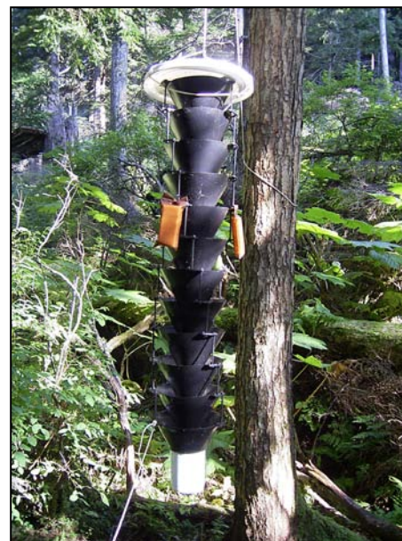
Funnel trap with ultra-high release "sponge" lure devices
