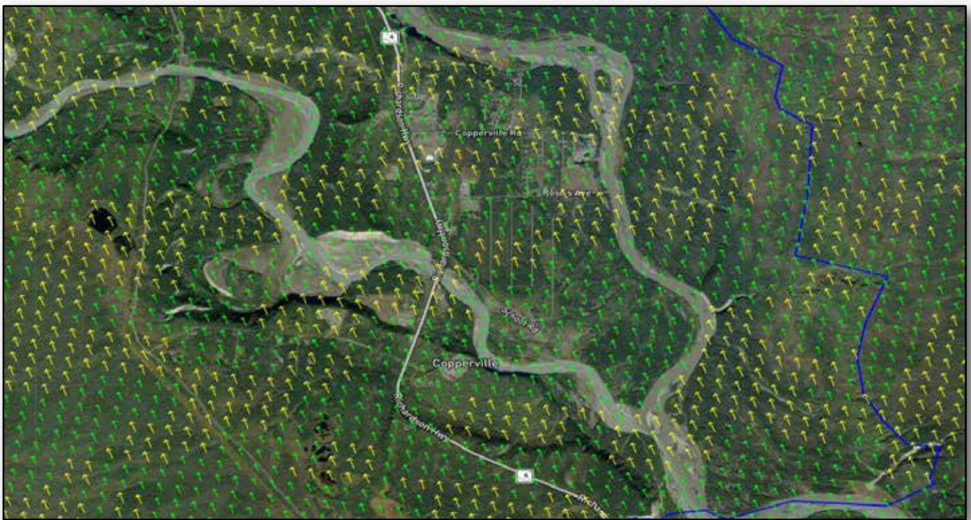
Page 6 of 12:: Terrain influences of wind speed and direction shown by arrow direction and color. See Page 2 for map legend. CWPP Boundary (blue). Wind speed 15 MPH and SE direction.
