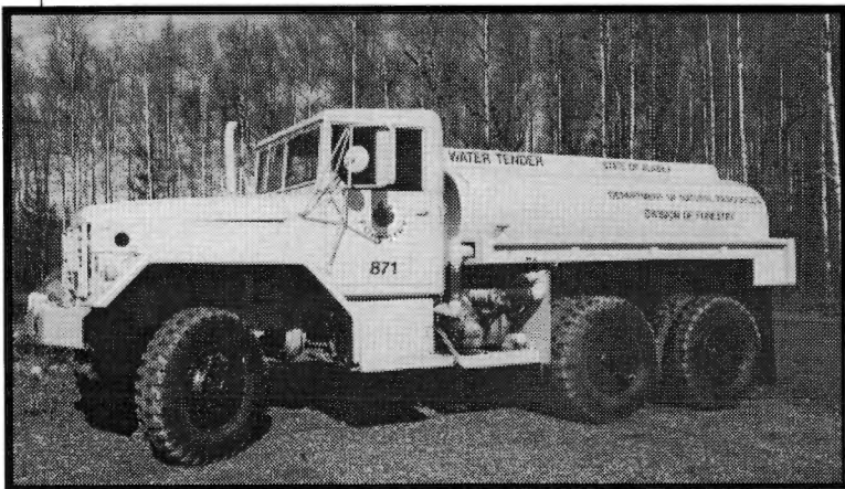
FEPP before and after. A 1,200-gallon water tender now refurbished and being used for wildland fire suppression. The cab and chassis is from a five-ton military dump truck and the tank is from a "deuce-and-a-half" military fueler. (M. Scott Christy)
