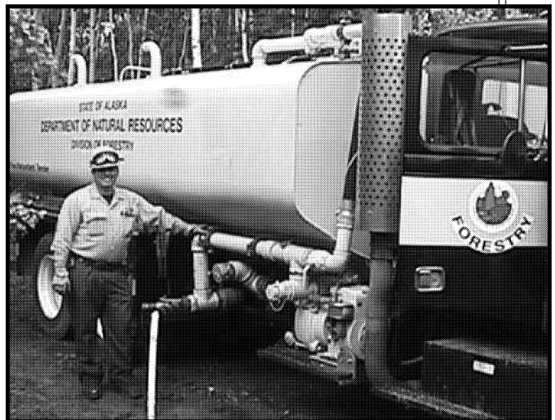
Eagle River shop staff created this water tender using the tank from a military fueller and a state surplus road sander truck chassis to which they added a water pump. The tender, operated by Geary Cooper of the Mat-Su Area, performed very well during the Clear Fire. (Scott Christy)
