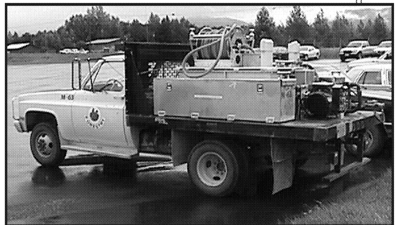
The division's shop in Eagle River converted this former military pickup truck (top photo) into a brush engine. The truck has a new volt system, heater, tires, siren, emergency lights and new paint. It carries a water pump, foam unit, hose reel and a 240-gallon water tank. (Scott Christy)
