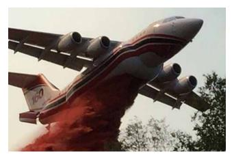
This RJ85 Aeroflite is a new generation air tanker, secured through a contract with the US Forest Service. It carries 3,000 gallons of retardant in a single load.
